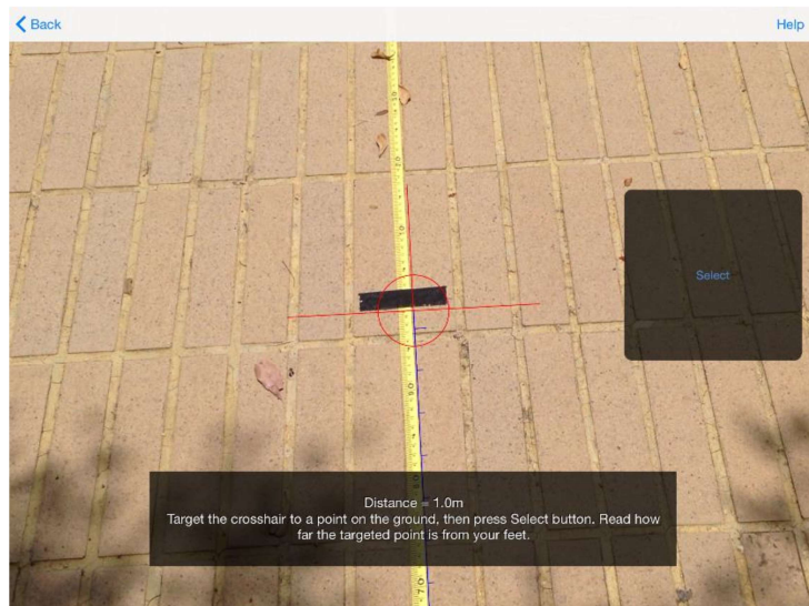
Figure 2 The line for pointing and numerical distances show on screen (Measure Tape HD application).
