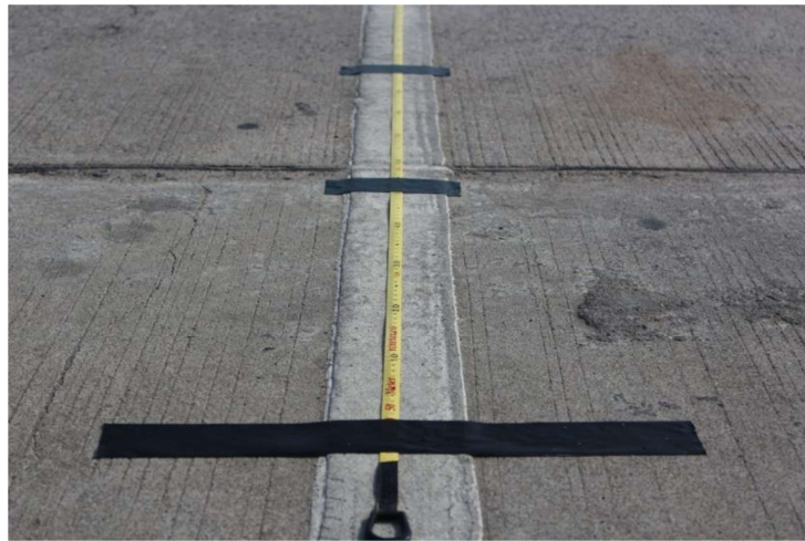
Figure 1 The black tapes set on the street in various distances along the fiberglass measuring tape.
