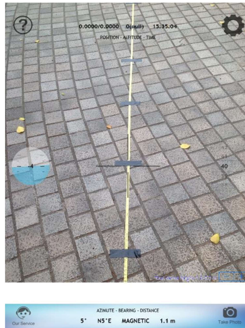
Figure 3 The line for pointing and numerical distances show on screen (iHandy application).
