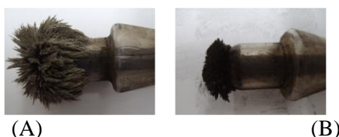
Figure 1. A. Attraction between nickel powder and magnetic applicator And B. attraction between cobalt powder and magnetic applicator
