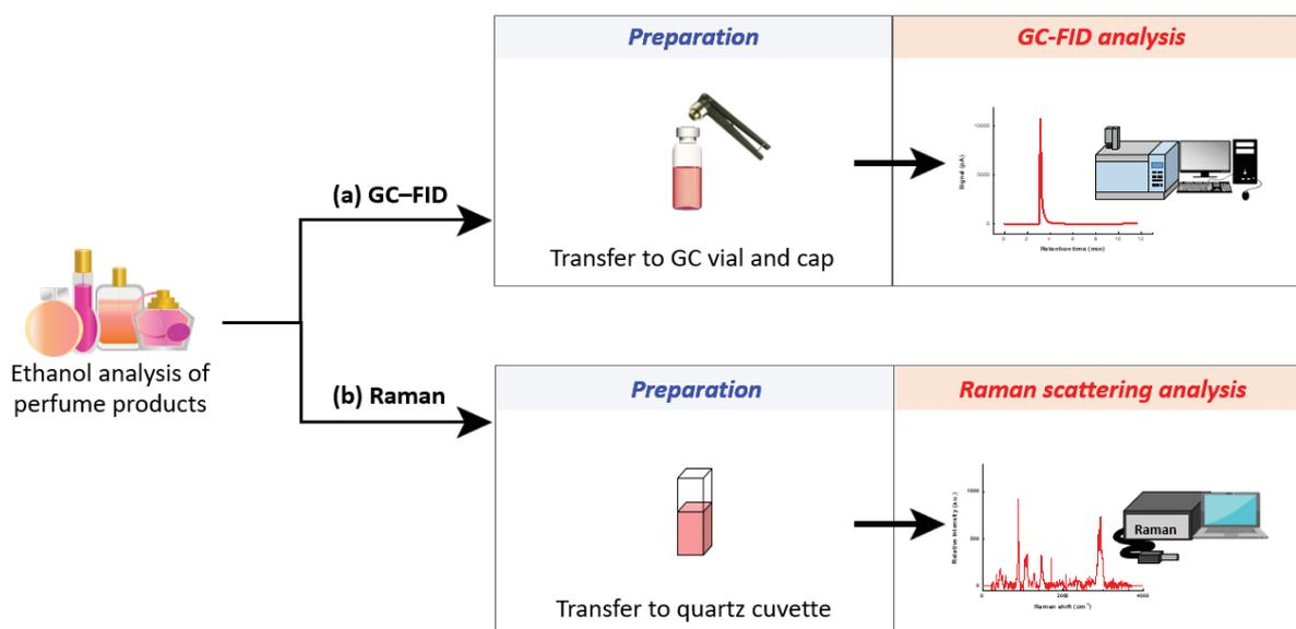
**Figure 2.** Schematic of ethanol measurement in perfume by (a) GC-FID and (b) Raman scattering.
