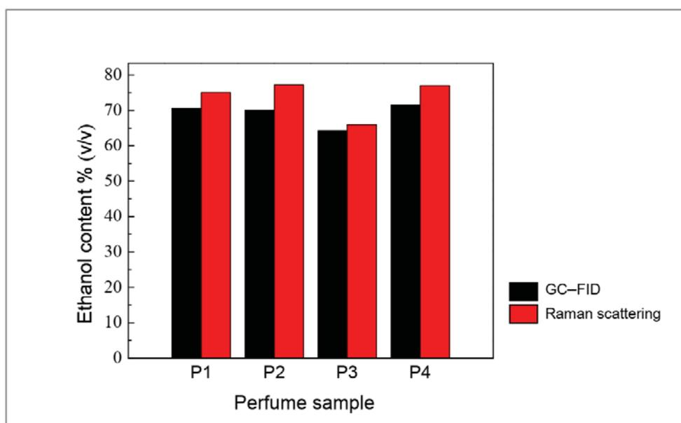
**Figure 4.** Bar graphs of measured ethanol contents in % (v/v) in four perfume products (P1, P2, P3 and P4) using GC-FID and Raman scattering.
