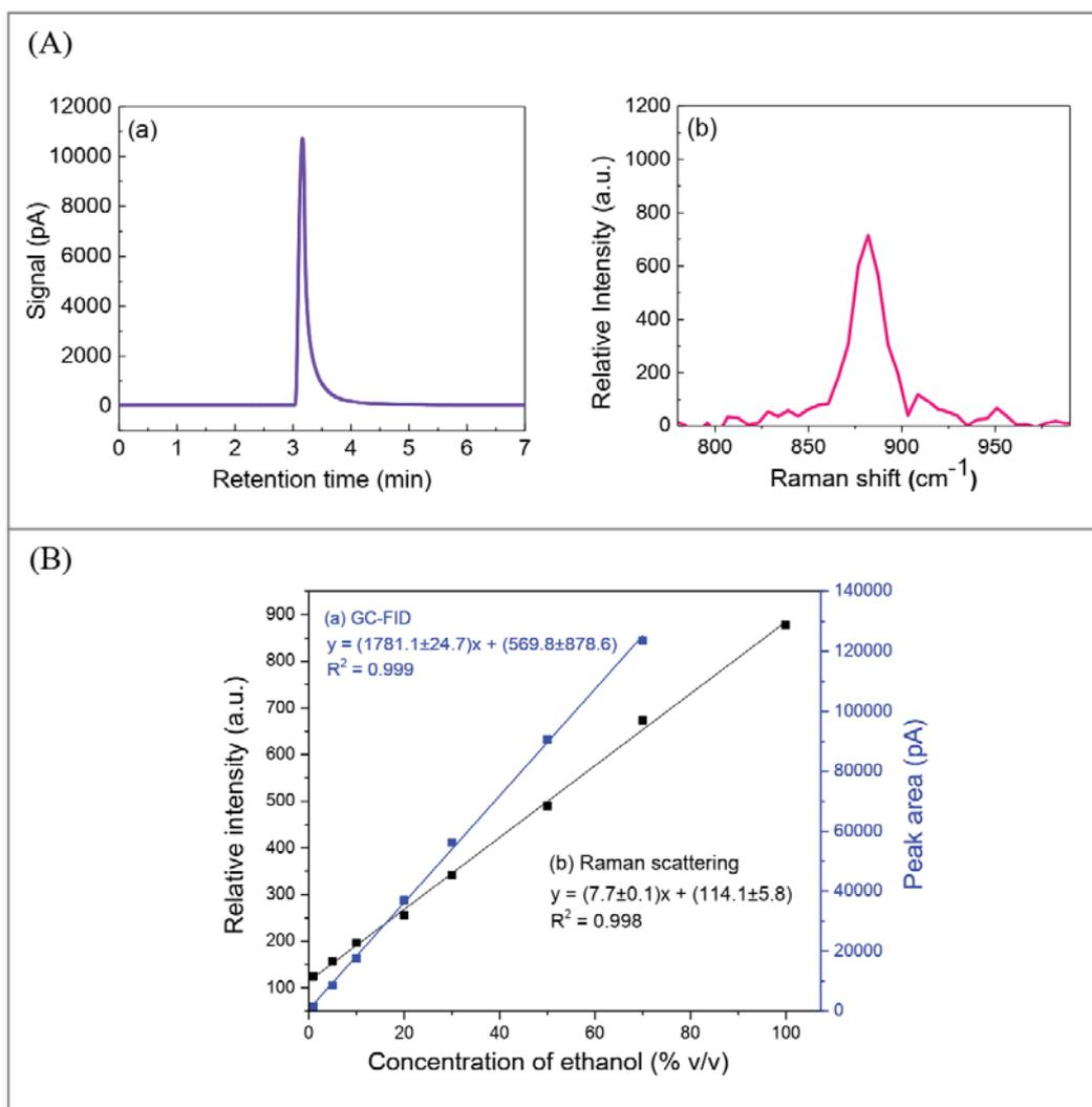
**Figure 3.** (A) An example of (a) chromatogram peak and (b) Raman scattering peak of ethanol at concentration of 70.0% (v/v). (B) Calibration curves of standard ethanol solutions for the two methods: (a) GC method, 1.0 – 70.0% (v/v) and (b) Raman scattering method, 1.0 – 99.9% (v/v).
